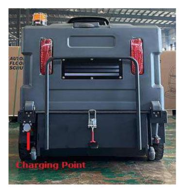
The charging point is located on the left side of the machine. Just plug the charger pin into the machine to charge as shown in the picture.
