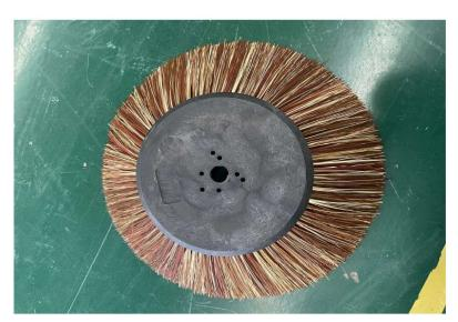
To replace the side brush, loosen the side brush flange locking screw, knock off the side brush flange, remove the fixing screws (4 M6 flange screws) between the flange and the side brush, replace the side brush with a new one, tighten the fixing screws, and brush the flange, and finally tight the screws.
