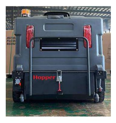
When you need to empty the hopper, first buckle the hopper bin upwards Pull away and then pull the hopper handle back to dislodge the hopper. The hopper is separated from the machine. After empty the hopper, aim the hopper mouth at the machine Slowly push forward in the correct position, push the buckle to the bottom and then Press down firmly to return the hopper to its place.
