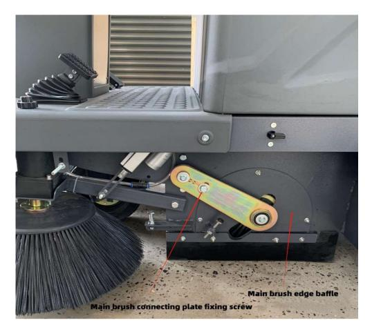
When it is necessary to replace or clean the main brush, open the left flap, unscrew the main brush connecting plate fixing nut, and drag out the connecting plate, then unscrew the main brush side baffle fixing nut, remove the main brush side baffle, and then the main brush side baffle can be removed. Brush out. After replacement or cleaning, install the main brush in the reverse order as described obove.
